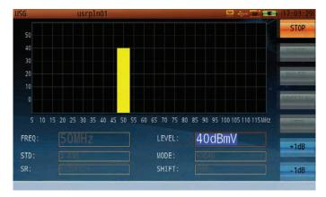
Figure 21: Upstream Signal Generator
