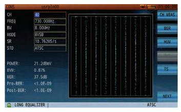
Figure 18: 8VSB Signal Demodulation
