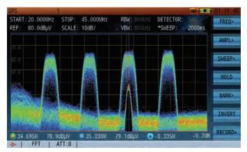
Figure 5: Persistence Shows Ingress Signal Under DOCSIS Upstream Signal
