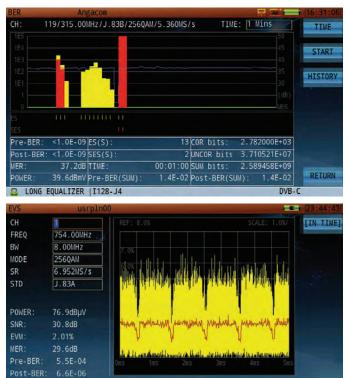
Figures 16, 17: EVS Locating Narrow- and Broadband Interference Signals
