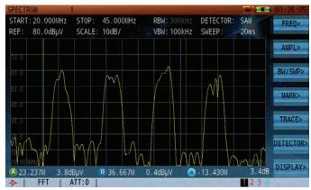
Figure 9: DVB-C Channel Measurement
