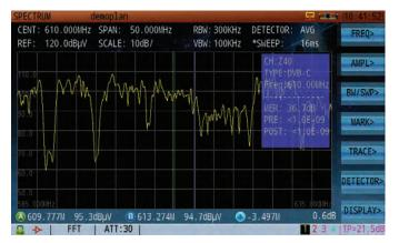
Figure 2: Simultaneous Spectrum and QAM Analysis
