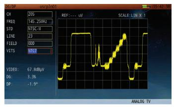
Figure 8: Analog TV Gated Measurement: Video Parameters
